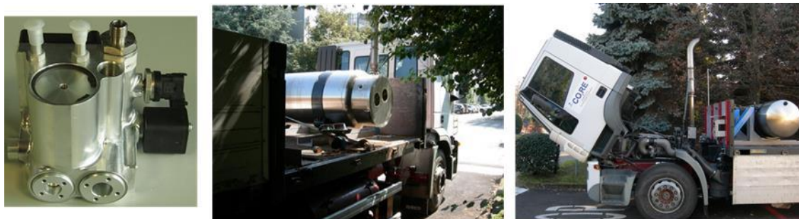
Fig. 20: Electronic Pressure Regulator (Proto C) and LNG + NG vehicle lay-out
