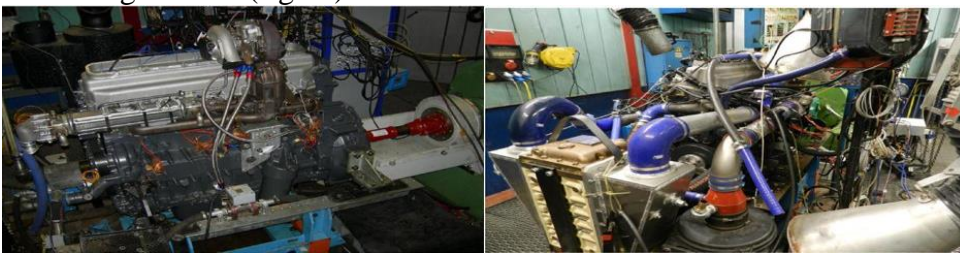
Figure 13: Diesel and NG prototypes on test bench
