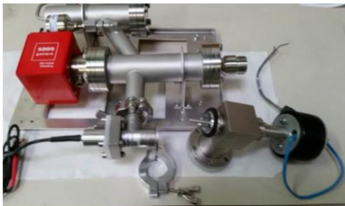
Figure 12: Left: scheme of the Sniffles vacuum system. Right: picture of the vacuum chambers during assembling.
