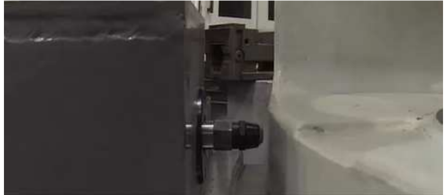
Figure10: Part positioning and the gap between the actuator and the part
