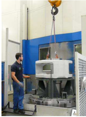
Figure10: Part positioning and the gap between the actuator and the part
