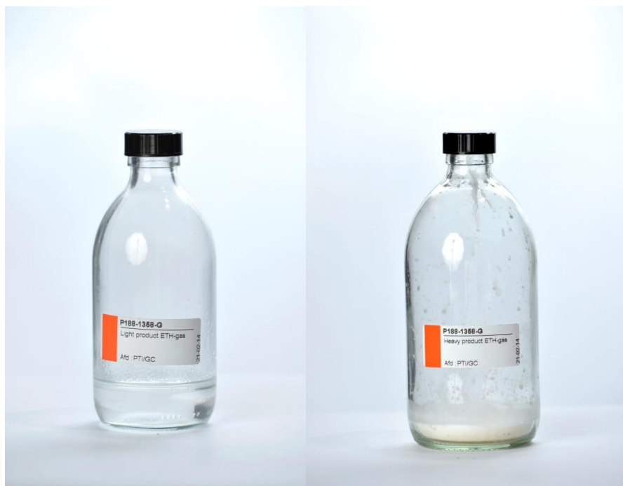
Figure 21: The light (left bottle) and heavy (right bottle) product produced during the Fischer-Tropsch run with the synthesis gas produced by the ETH. The heavy product is a solid white wax. The liquid product consists of mainly water with a thin layer of liquid hydrocarbons floating on it.
