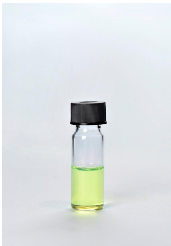
Figure 22: The liquid product produced after hydrocracking the Fischer-Tropsch wax (the heavy product shown in Figure 21).
