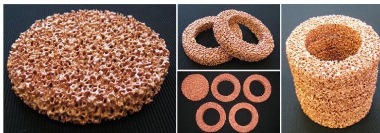
Figure 6: CeO 2 RPC parts fabricated for the solar cavity-receiver. One set consists of a disk (20 mm thickness, 100 mm OD) and four rings (20mm thickness, 60 mm ID, 100 mm OD).
