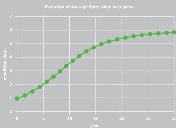
**Figure 5:** Some impressions of components in the SCBA framework: scheme depicting monitoring data input towards maintenance strategy (top right), simplified example of decision tree for maintenance scenarios (top left), degradation function based upon Markov transition matrices (left), differentiation into different costs (bottom) and Net Present Value results of a maintenance scenario based upon an alternative monitoring device (right).
