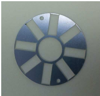
View of the part designed to hold and align the cantilevers inside the gas cell
