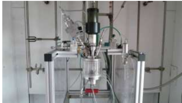
Figure 2 – glass reactor used (P up to 10bar)
