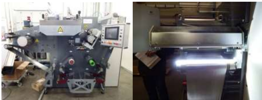
Figure 1: Start-up trials with aluminium current collector foil (left), application area and precompacting unit (middle), trials with carrier foil made from polyimide (right), monitoring system (In-Core technology) installed at demonstrator
