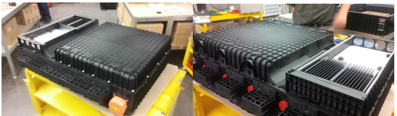
Figure 4 :High-level integration means the set-up under the vehicle is ensured with the fastening on the frame and the plugging of 4 connectors.
