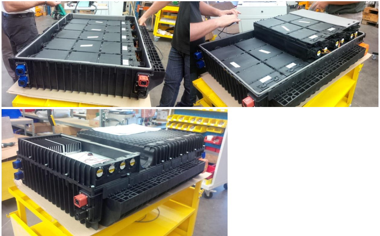
Figure 3: The 2-layer concept, required to ensure the 18kWh energy storage in the bulking with the size of the chosen cells, leads to a modular conception
