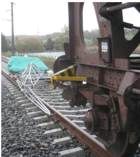
Figure 19: Benkelman beam for the measurement of track elastic deflection
