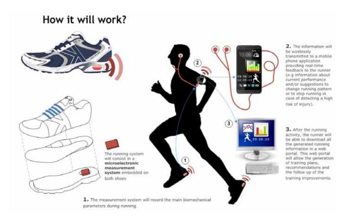
The running system will consist in a **microelectronic measurement system embedded on both shoes**, able to gather and transmit the main biomechanical parameters during running.
