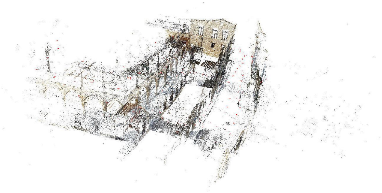
Figure 31: Adjusted camera positions and reconstruction for over 1000 images of old University building in Nicosia (Cyprus).
