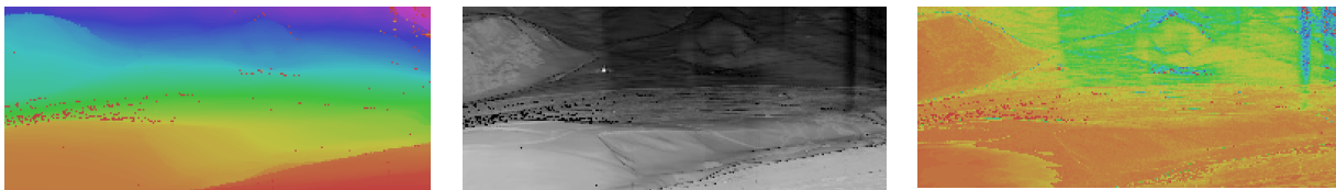
Figure 35: Alpe Rauz example for target scan performed on 01/28/2014 17:00. Reflectivity (bright: good reflectivity, dark: bad reflectivity).
