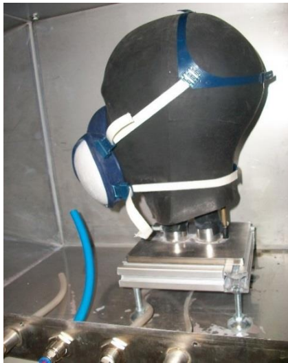
Figure 13a. Sheffield head detail, and Sheffield head perform – RMM testing
