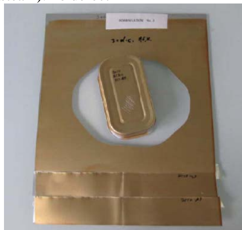
Fig. 20: Test using Formulation C applied on Aluminium
