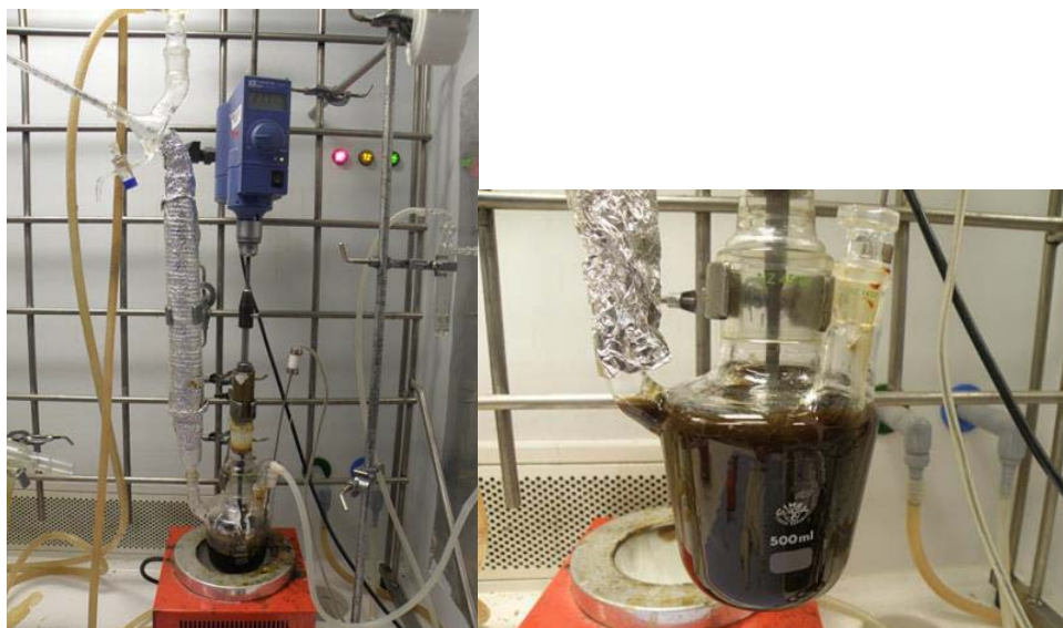
Fig. 12: Laboratory apparatus for polycondensation reaction used for synthesis of cutin based polyester.
