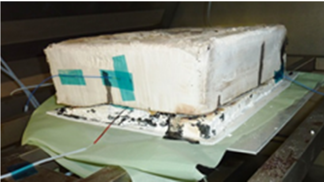
Figure 10: Final tool assembly prior to processing. Thermocouple probes can also be seen
