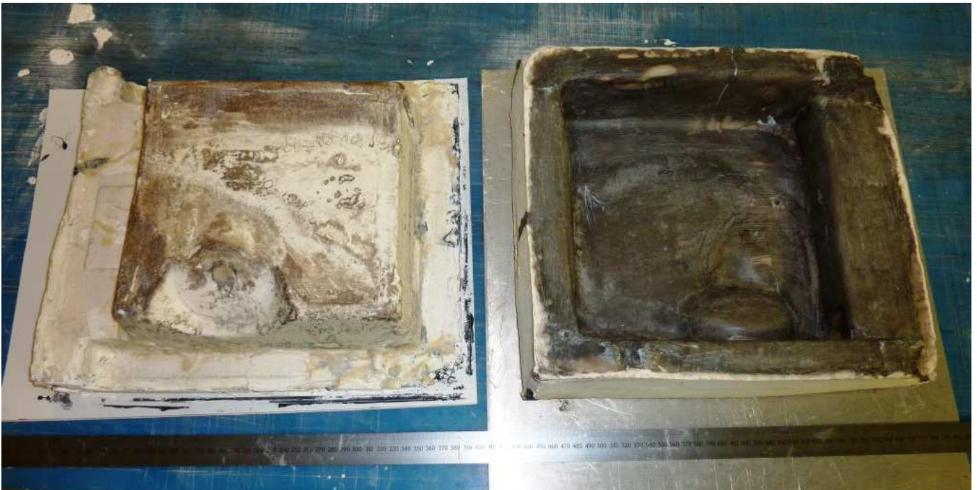
Figure 30: Plug (left) and cavity (right) tools. The blackened areas are the wax remains after the production process
