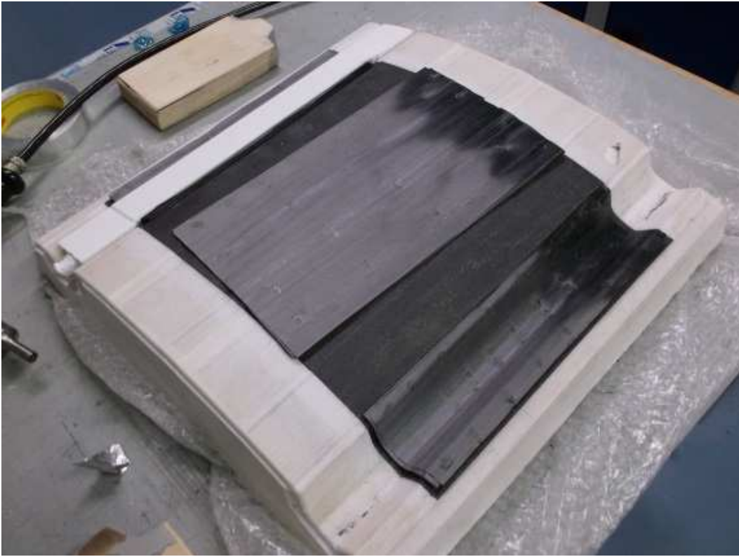
Figure 17: Carbon fibre PEEK prepreg being formed on the tool
