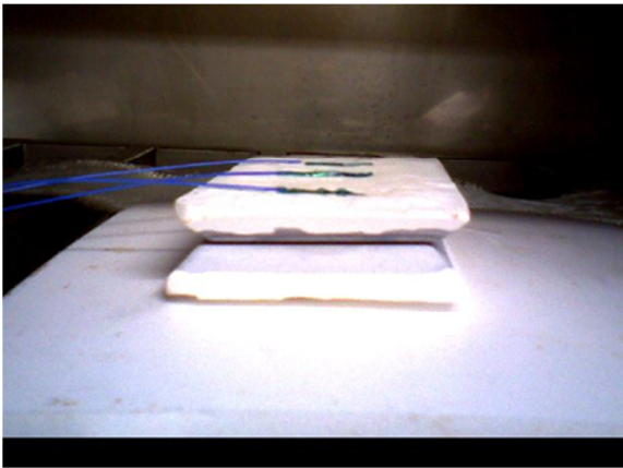
Figure 15: Tool layout after completion of the PEEK polymerisation reaction – side view
