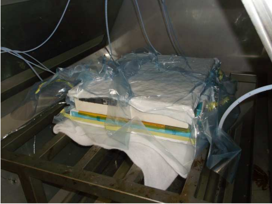
Figure 19: Tooling under vacuum and ready to be MW processed
