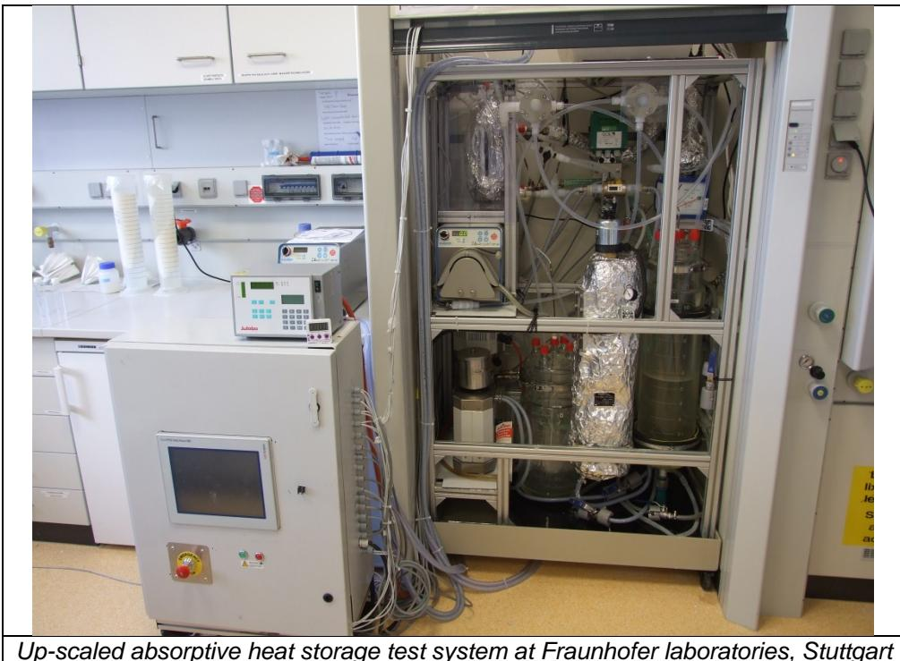
*Up-scaled absorptive heat storage test system at Fraunhofer laboratories, Stuttgart*
