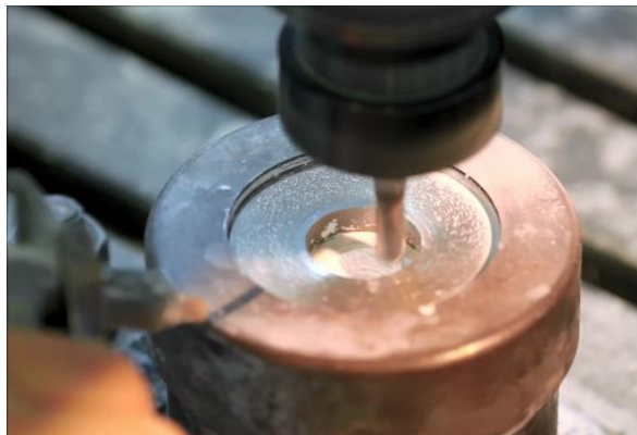
Figure 10 Machining of the internal face of the ceramic cup once it is subjected with the metallic device
