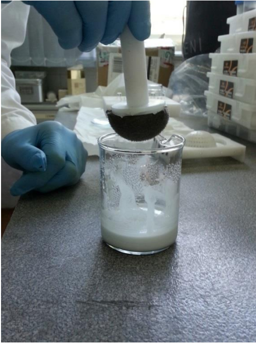
Figure 27 Soaking of the ceramic cup coated with the dense layer and by a PU sponge
