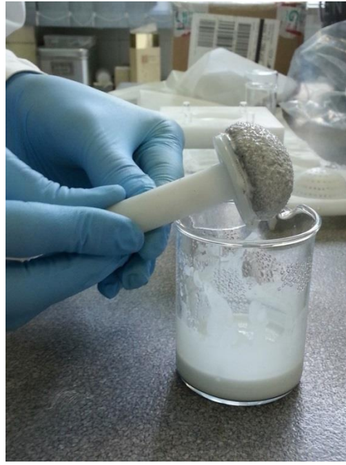
Figure 27 Soaking of the ceramic cup coated with the dense layer and by a PU sponge
