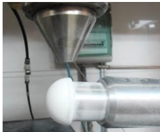
Figure 24 Dense coating realisation on the ceramic cup by laser cladding (AIMEN)
