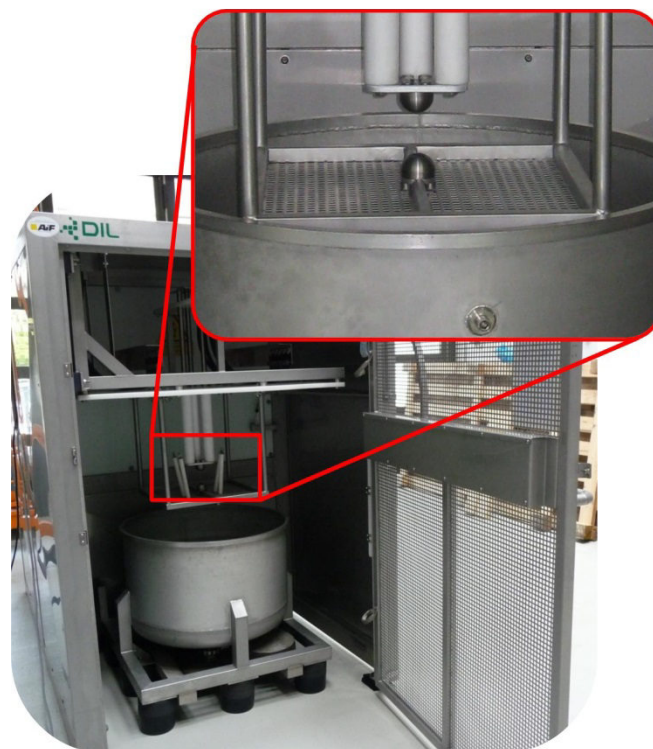
Figure 2.3. Shockwave prototype intended for meat tenderization developed within a German-funded research project, AiF-15884 N (2008-2011).
