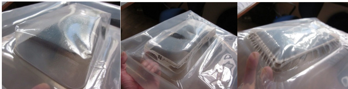
Figure 4.2: Results of the deep drawing process of the potential thermoforming TPU based film.
