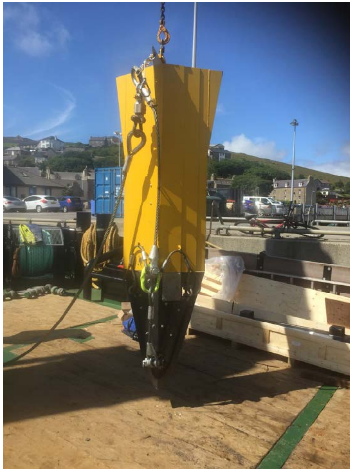
Figure 15 Assembled anchor/follower with bridle arrangement at EMEC (without guide frame)
