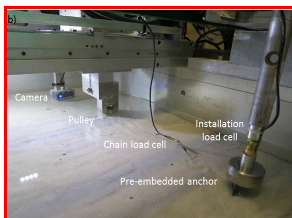
Figure 10: Geotechnical centrifuge at UWA, showing embedment test set-up (bottom left) and capacity arrangement (bottom right).
