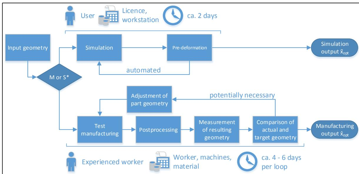
Figure 1: Comparison of workflows for the manufacturing-based and the simulation-based process chain. Both share the initial geometry as input and an optimized geometry as output in order to manufacture a part without dimensional deviations in respect to the initial geometry. The necessary staff, the respective sources of expenses and the expected time frame are given (Source [1]). \*M(achine-based) or S(imulation-based)
