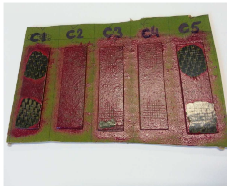
Figure 5: Test samples used in the paint adhesion test (evaluated using the cross-hatch technique)
