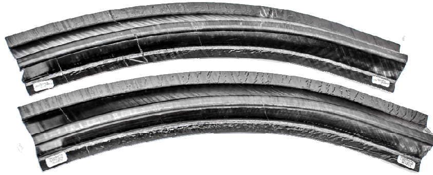
Figure 5 Feasibility article stiffeners upon thermoforming laminates with steered 0° plies and standard blank (below)
