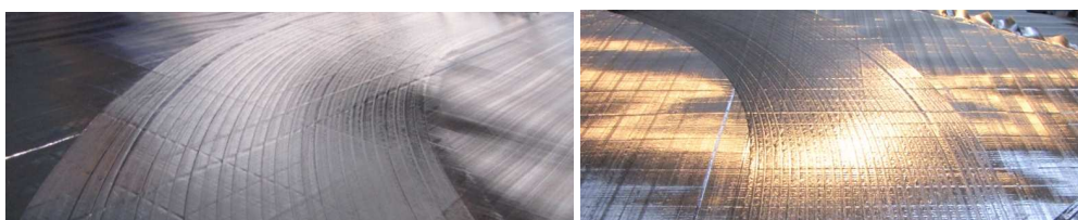
Figure 4 Steering of 0^\circ plies along the curvature of the feasibility article during TFP
