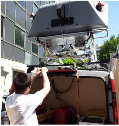
Figure 54 GNSS/INS benchmarking setup
