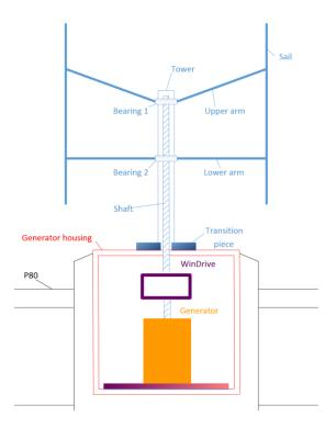
Figure 20. Direct coupling of the VAWT shaft with a generator
