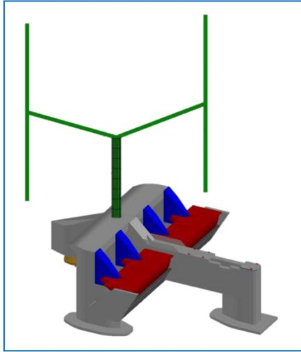
**Figure 7. Initial concept of the hybrid VAWT-WEC device**
