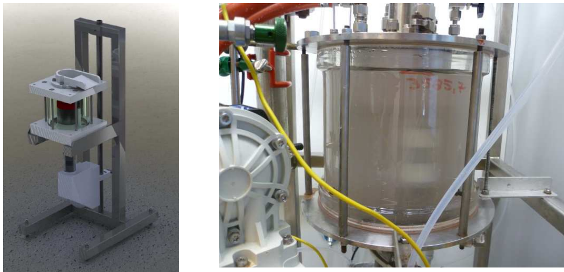
Figure 11: Left - Freeze crystallizer set up design; Right – Freeze crystallizer filled with fermentation broth containing IA.
