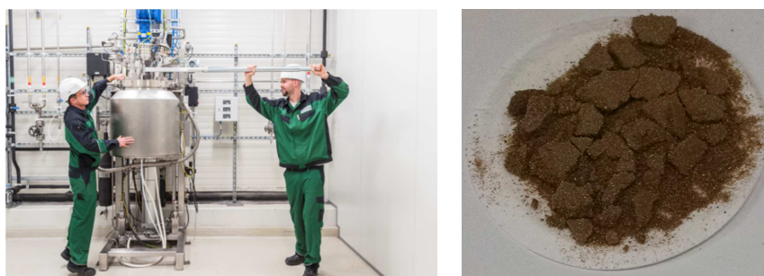
Figure 14: equipment used for super heat crystallization at bench scale and crystals obtained after purification with this technology (purity obtained here is ~95 %wt).
