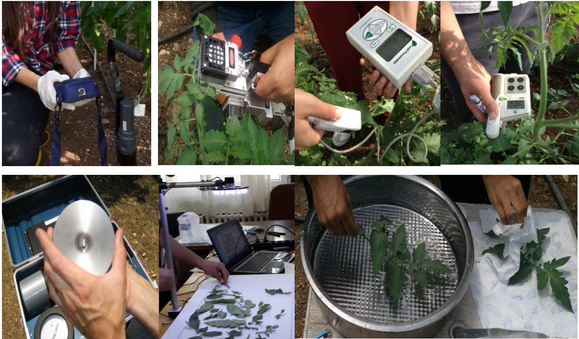
Figure 14. Soil water content, photosynthesis, stomatal conductance, SPAD, leaf water potential, leaf area and relative leaf water content measurements.
