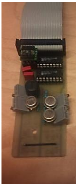
Figure 8. A real life image of the 4 MOS sensors, temperature sensor and humidity sensor developed to quantify SCFA on line inside the body or gut simulation models.
