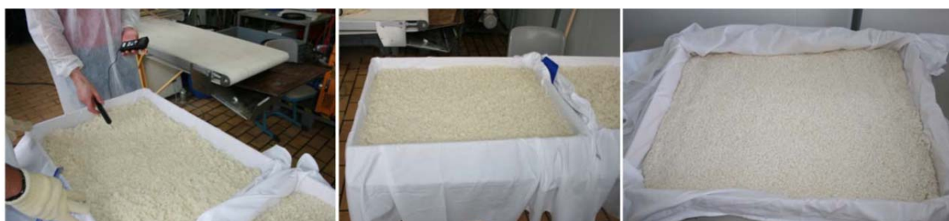
Fig.: Preparation of trays for 50 kg Solid State Fermentation (NST)
