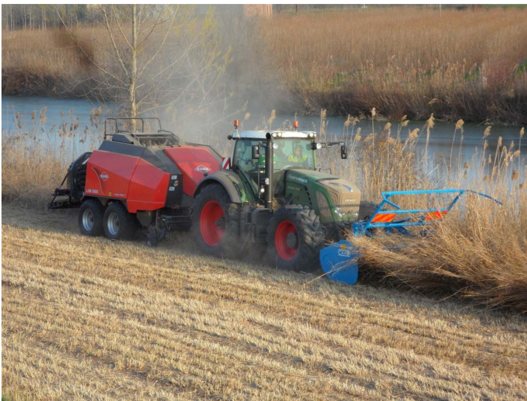
Figure 6 – SPAPPERI. Harvesting yard on Arundo donax L. composed by mulcher and baler; the biomass is collected only in one tractor passage. http://www.nobili.com/en/cat_serie.php?ID=411
