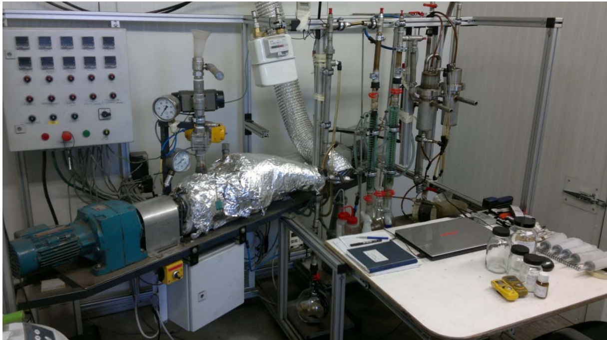
Figure 3 – BTG. Photograph of the torrefaction setup
