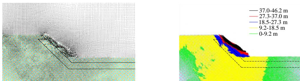
**Figure 4.** CFD-DEM analysis of a submarine landslide triggered by thermal dissociation of methane hydrate.
