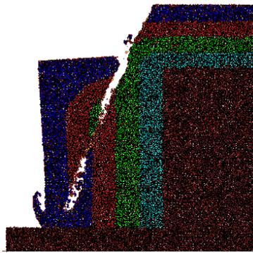
**Figure 1.** DEM simulation of a rock slide as a result of weathering.
