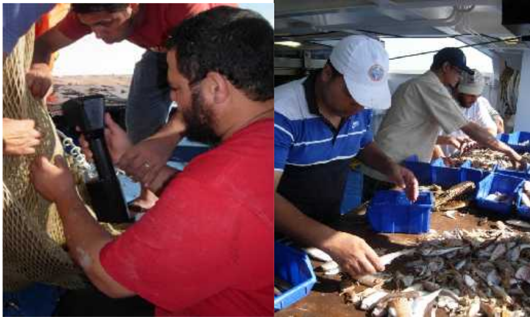
Figure 14: On Board “FORCE participants during the measurement of the codend mesh opening with the electronic gauge and sorting of fish”.
