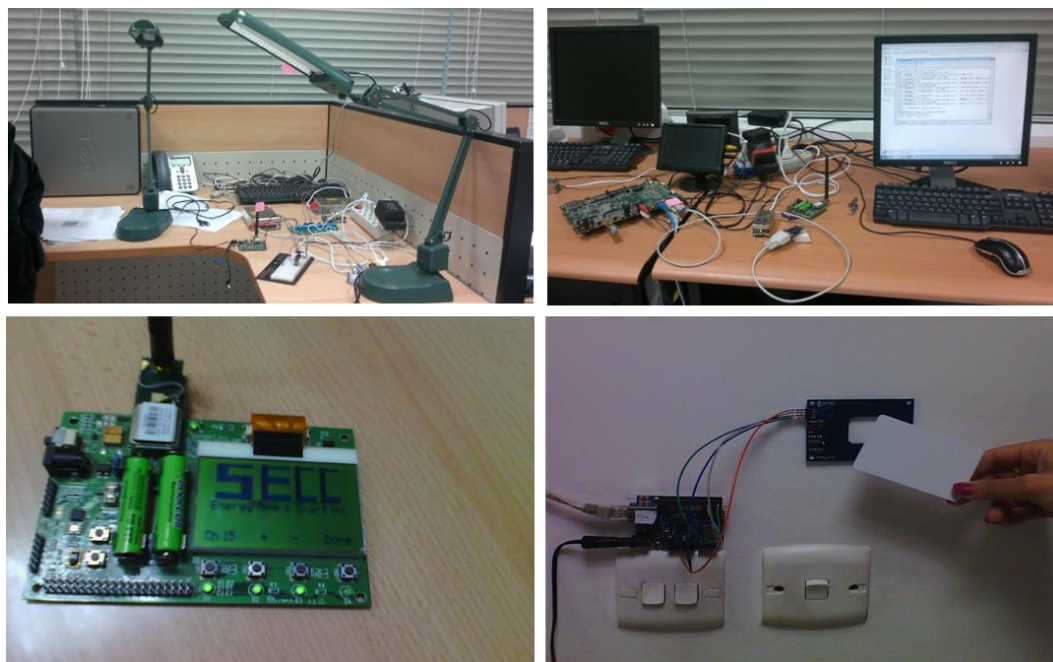
Figure 2 - Controlling light (upper left), multimedia playback (upper right) via Zigbee node after receiving commands from Zigbee coordinator (lower left) based on user identification using RFID (lower right)
