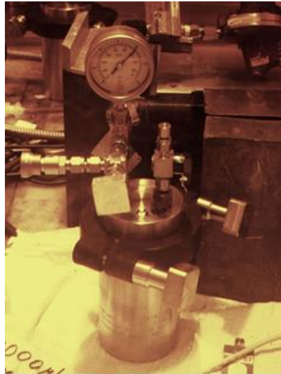
Figure 5: Dissolution based release experiments conducted under hydrogen pressure.
