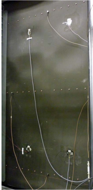
Fig. 5: Panel 1 reference – skin side view to the panel with buckling waves (70% of predicted failure load).
