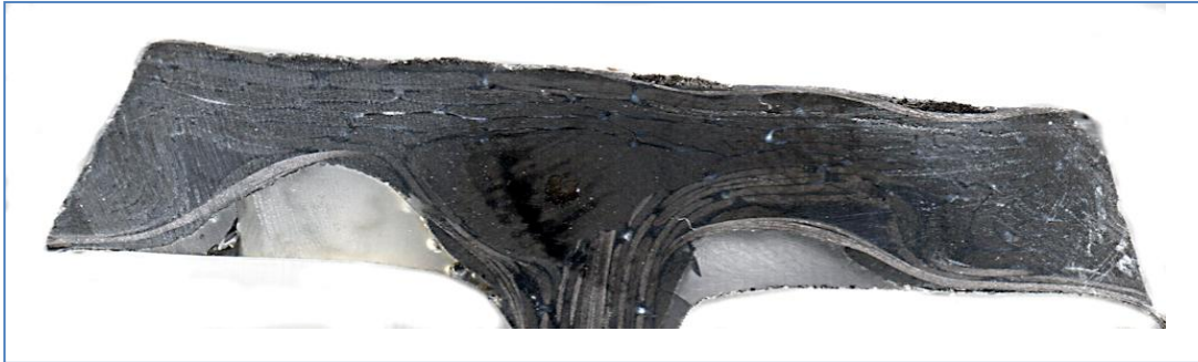
Figure 14 :Macrographs of the cross section cut out of the demo part showing major defects
