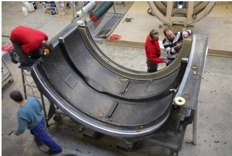
Figure 11 : The fiber preform inside the tool
