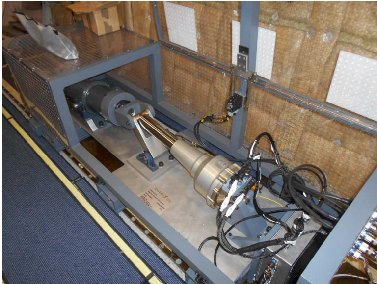
Image 1. ARMLIGHT EMA actuator performing tests at ATR aircraft flight demonstrator
