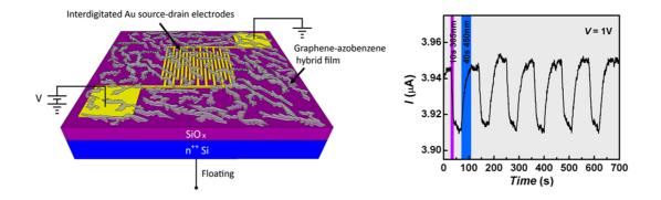
**Figure 1.** Left side: Scheme of the device configuration used for the characterisation of the organo-graphene hybrids. Right side: Optical modulation of device current response illustrated for a static bias and dynamic alternating UV and visible light irradiation.
