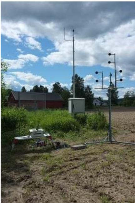
Figure 1: Microphone array in situ during a measurement campaign near Oslo airport.
