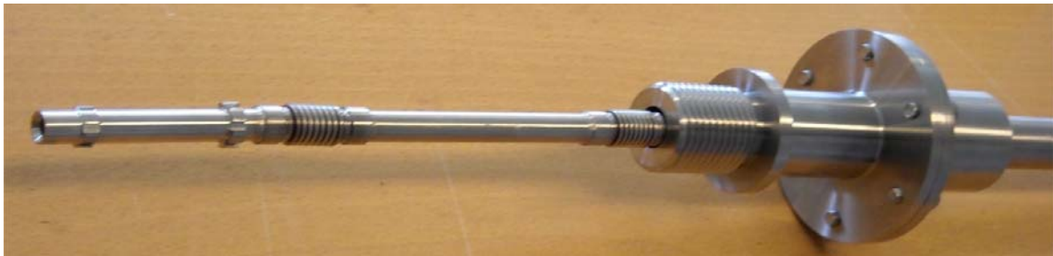
Figure 17: KEMA boroscope pyrometer with refractive optics
