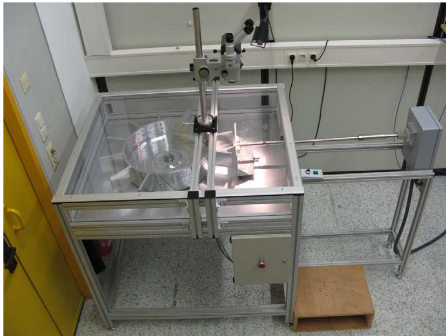
Figure 47: Rotating rig with mm-wave probe
