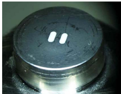
Figure 44: Sensor tip with sealed antenna
