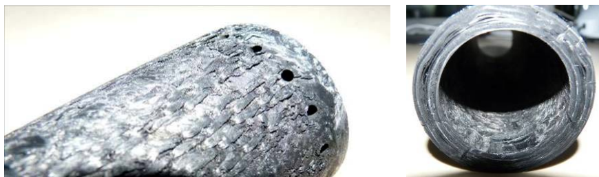
Figure 32: PSR-CMC liner machined for joining with the microfibre shells
