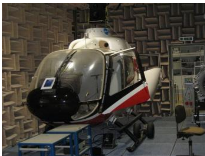
Figure 22: BO 108 mock-up in reverberation room
