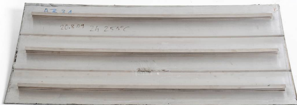
Figure 79: Creep formed panel made from AZ31 sheet and AZ31 stringers joined by LBW; Longitudinal joints realized by FSW.
