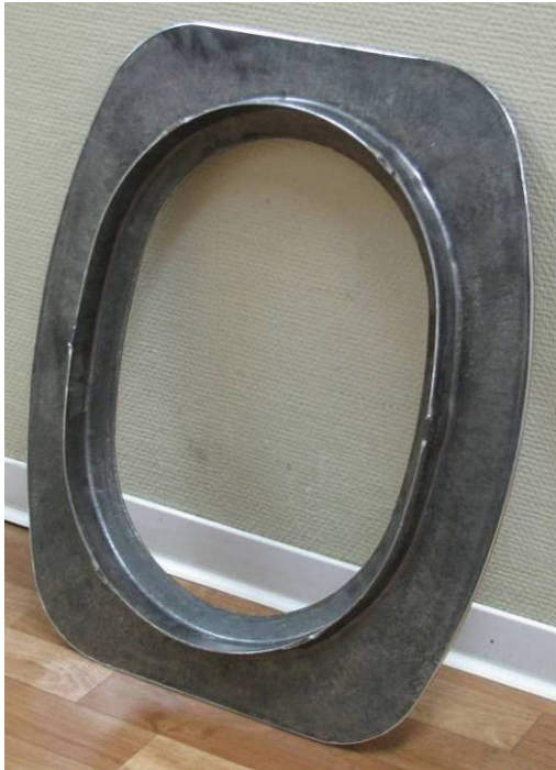
Figure 6: Window frame forging (flash removed)
