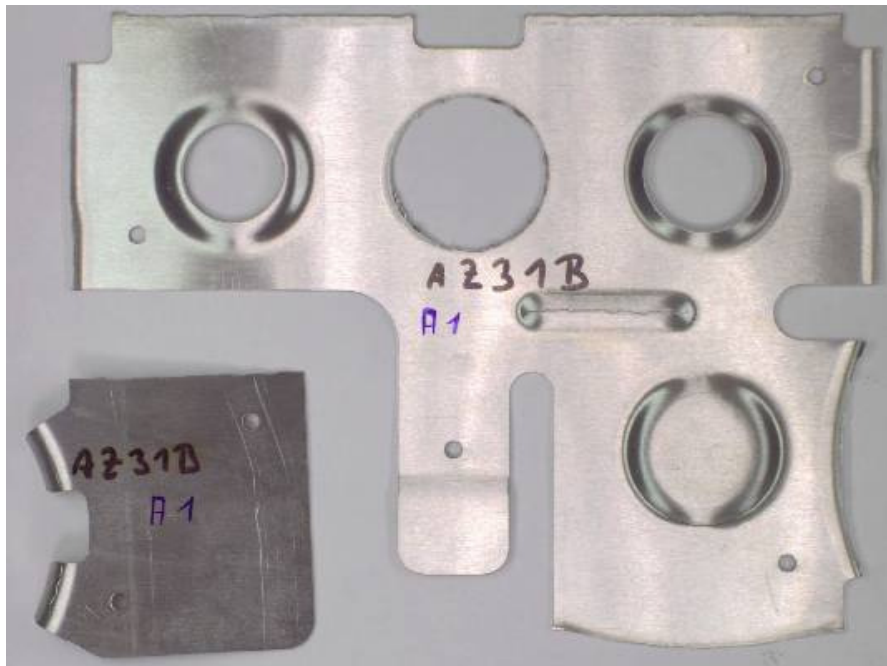
Figure 41: AZ31B (2 mm) part with broken flanges, crimps and cracks
