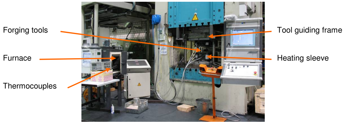
Figure 7: Forging tool of compressor wheel
