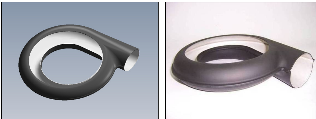
Figure 26: The compressor scroll, 3D solid model designed by LTS (left) and Final shape produced by PALBAM-AMTS (right)
