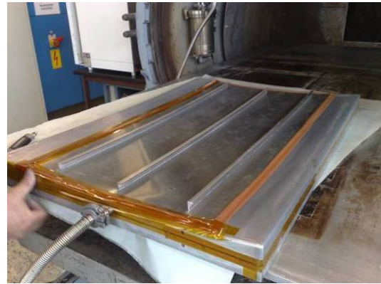
Figure 65: Creep formed demonstrator panel fixed in the tool
