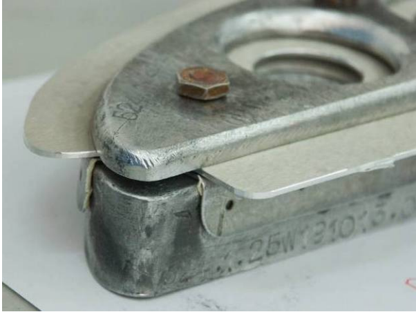
Figure 35: ZE10A-F placed on pad-formed Aluminium sheet to enlarge bending radii
