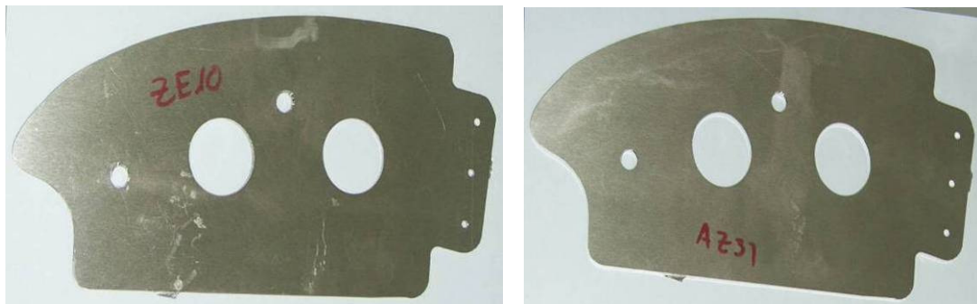
Figure 29: Magnesium flat patterns sheet after milling ready to be pad-formed, (left) ZE10A-F; (right) AZ31B-H24
