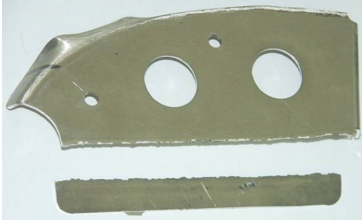
Figure 38: Unsuccessful pad-forming of AZ31B-H24 with the enlarged radii
