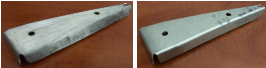
Figure 33: Comparison between original Aluminium test part (left) to Magnesium part (right)
