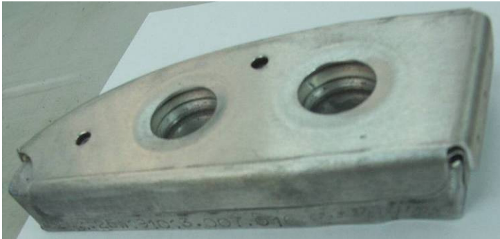
Figure 36: ZE10A-F after success pad-forming on Aluminium sheet (final radii of R3.5)
