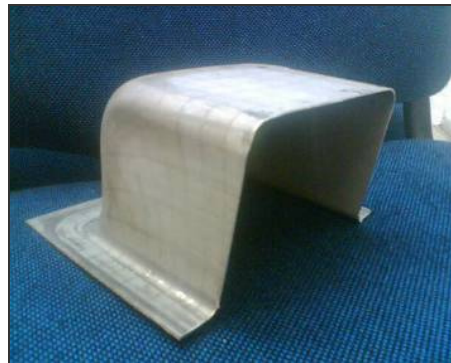
Figure 15: Experimental part model (left) and deformed Magnesium part (right)
