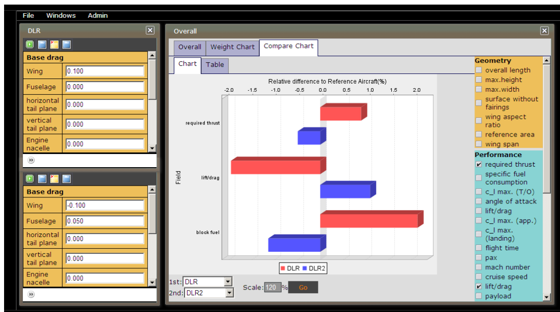
Figure 3 Presentation of the results comparing influence of different technologies to the reference aircraft performance. Here shown are the attributes thrust, lift over drag and block fuel
