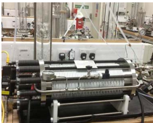
Fig. 26: 20 cell stack made and tested using down selected materials from partners. (ITM)
