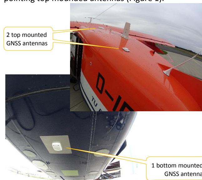
Figure 1 Multi-antenna set-up for novel aircraft on-board jamming mitigation solution
