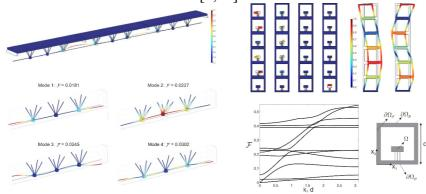
Spectral analysis of Bloch waves in a periodic elastic waveguide determine the dynamic response of a slender but finite structure such as a multispan bridge. Application to the "dancing bridge" in Volgograd, Russia, and the S'Adde bridge in
