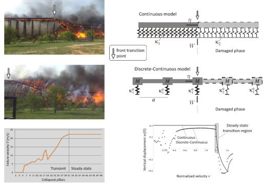
Analysis of slender discontinuous bridge structures has been examined considering the propagation of transverse waves in a two-dimensional elastic strip with
