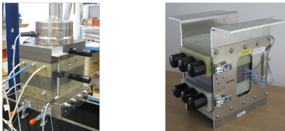
Figure 14. Compression test set-up for single cell compression with force and way sensor (left), MT-PEM Short stack with 8 cells (right)
