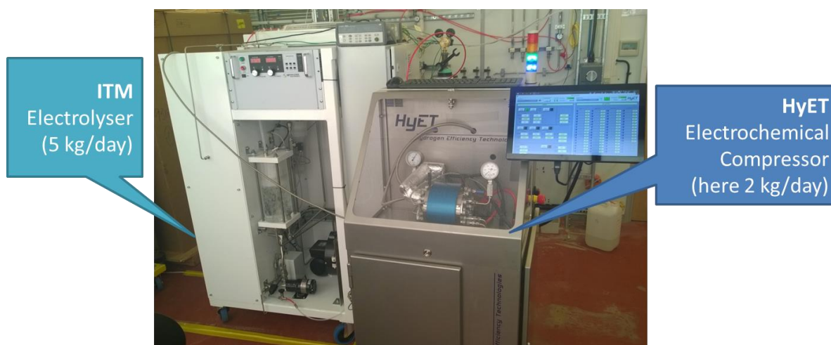
Figure 6 – Picture showing world's first integration and validation of the PEM Electrolyser and the Electrochemical Hydrogen Compressor (MoHyTO) in the field at ITM laboratory in Sheffield.
