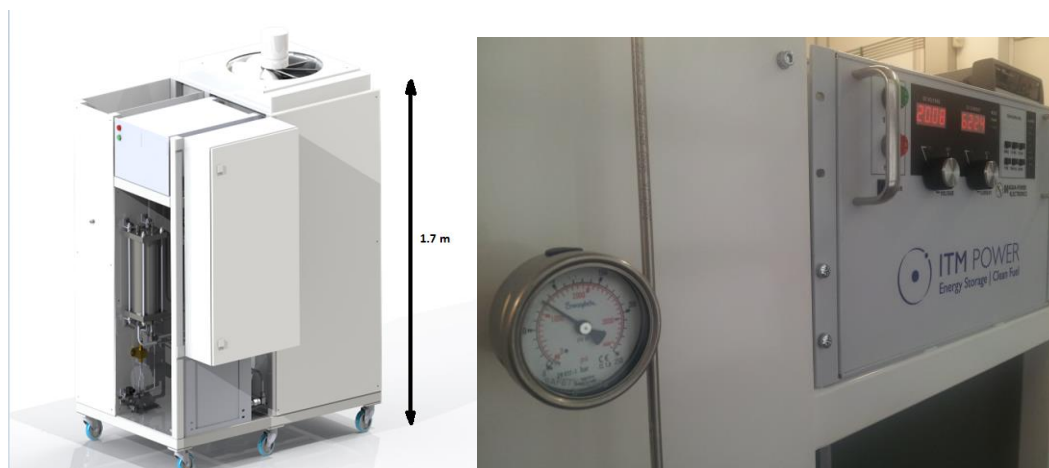
Figure 3 - 5kg H 2 /day, 80 bar PEM electrolyser achieving assessment criteria of 1.5 A/cm 2
