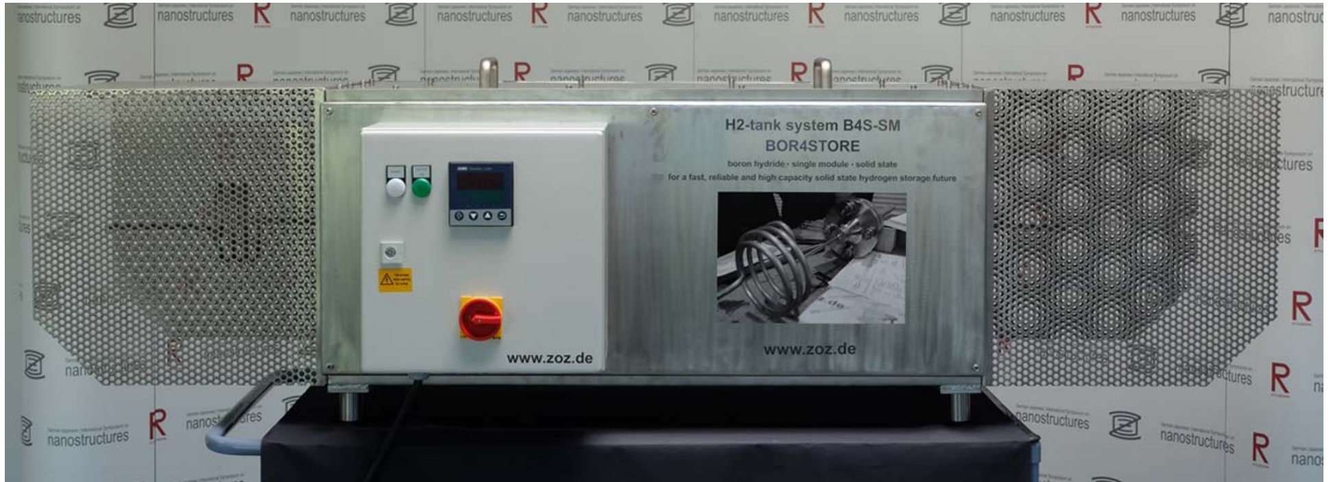
BOR4STORE single module tank (ZOZ name B4S-SM). Left and right heat shieldings for hydrogen supply and take-out line (left) as well as thermocouple lines (right). Image on heat shielding box shows cooling spiral in hydrogen line and flange of proper tank module
