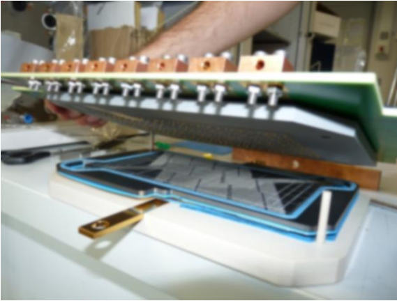
Figure 7: Complete cell setup with upper isolation plate containing holes for the contact pins.
